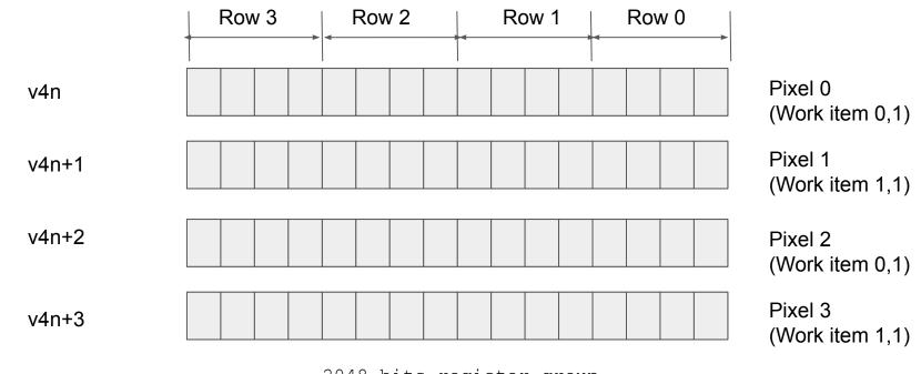
2048 bits register group vtype: VLEN=512 bits, LMUL=4 regs, SEW=32 bits
